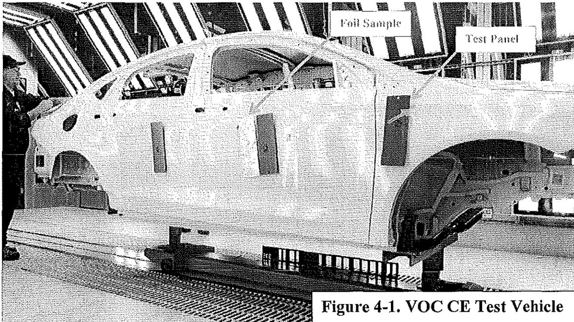
**Figure 4-1. VOC CE Test Vehicle**
