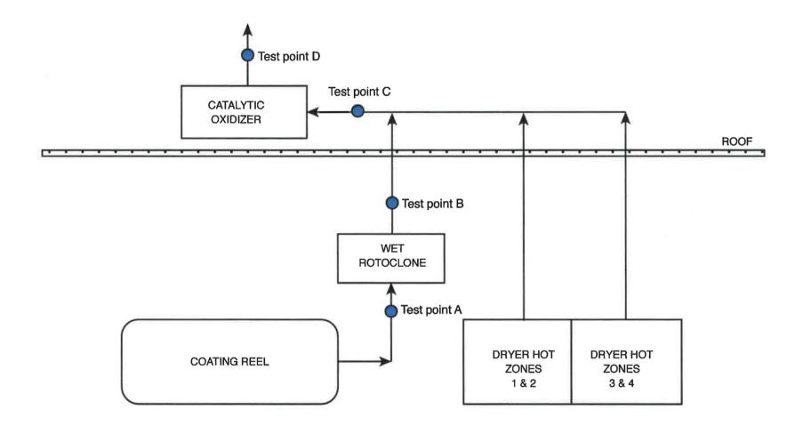
Test sites for VOC and volumetric flow rate
