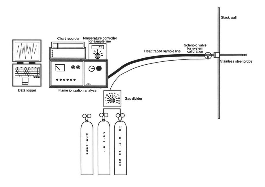
Figure 3.3 USEPA Reference Method 25A measurement system
