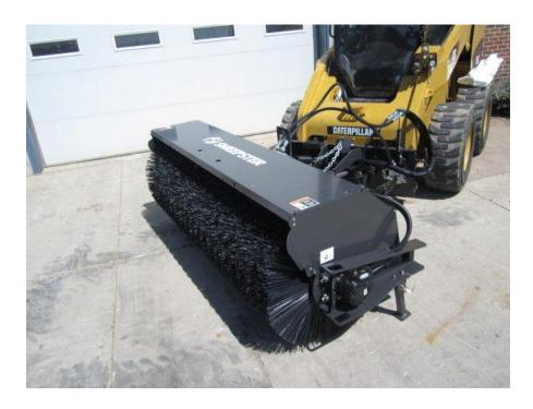
FRC yard is swept as needed with a sweepster power broom attached to a CAT 242b skid steer very similar to the one pictured above. The yard is only swept after it has rained or been watered down to minimize dust.
