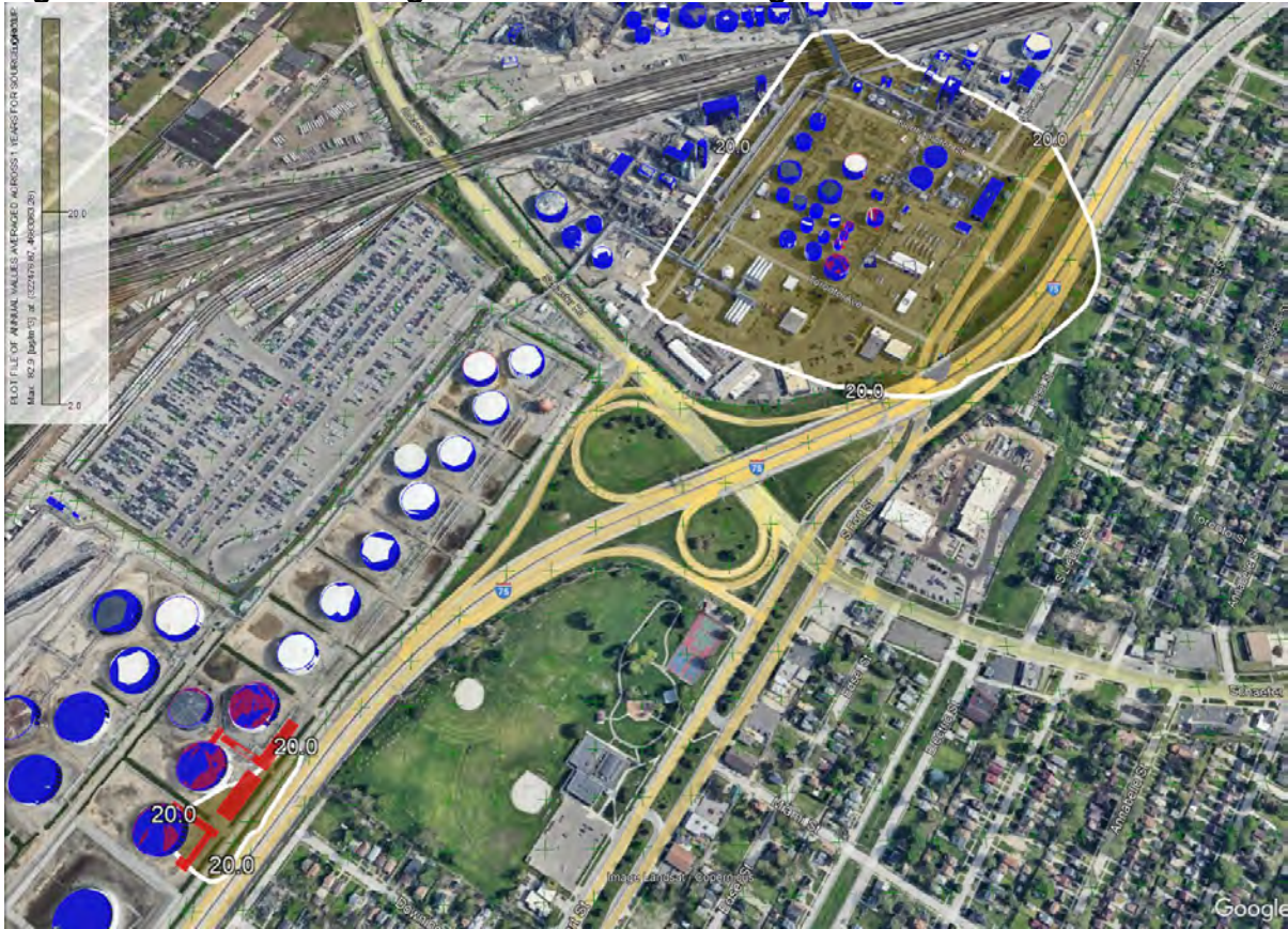
Figure 2: Gasoline Modeling Result with the Existing MPLX VRU Stack
