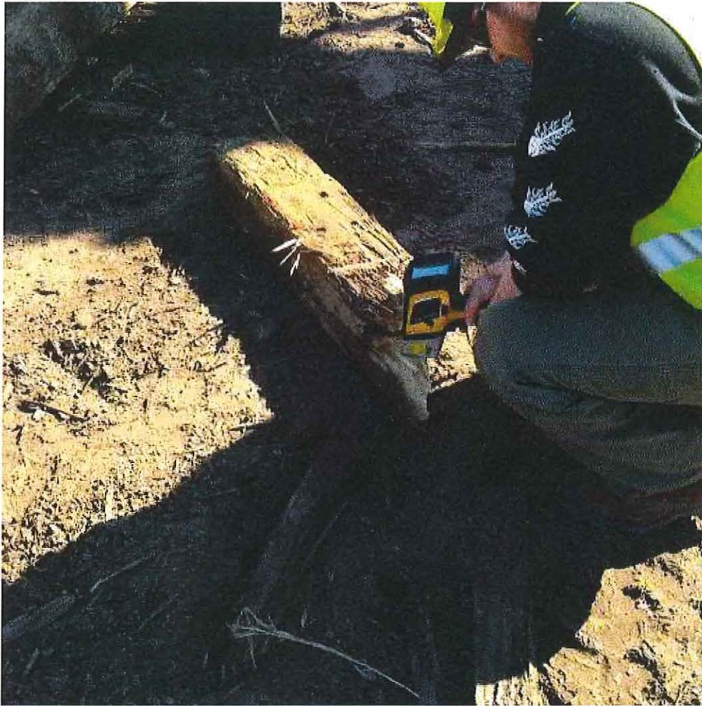
Image 2(XRF of Tie #3) : MA Energy employee using an XRF to monitor the chlorine content of the interior of Tie #3.
