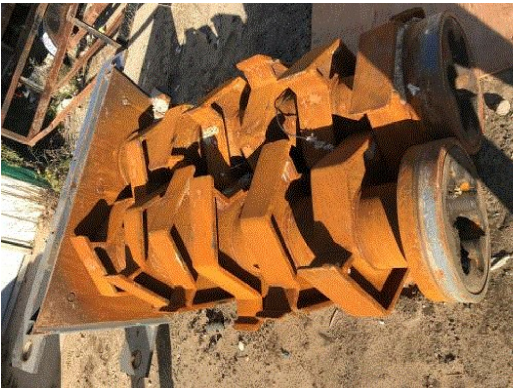
Image 6(Nonaggregate shaft) : Nonaggregate shaft with welds and weathering 9/4/2020
