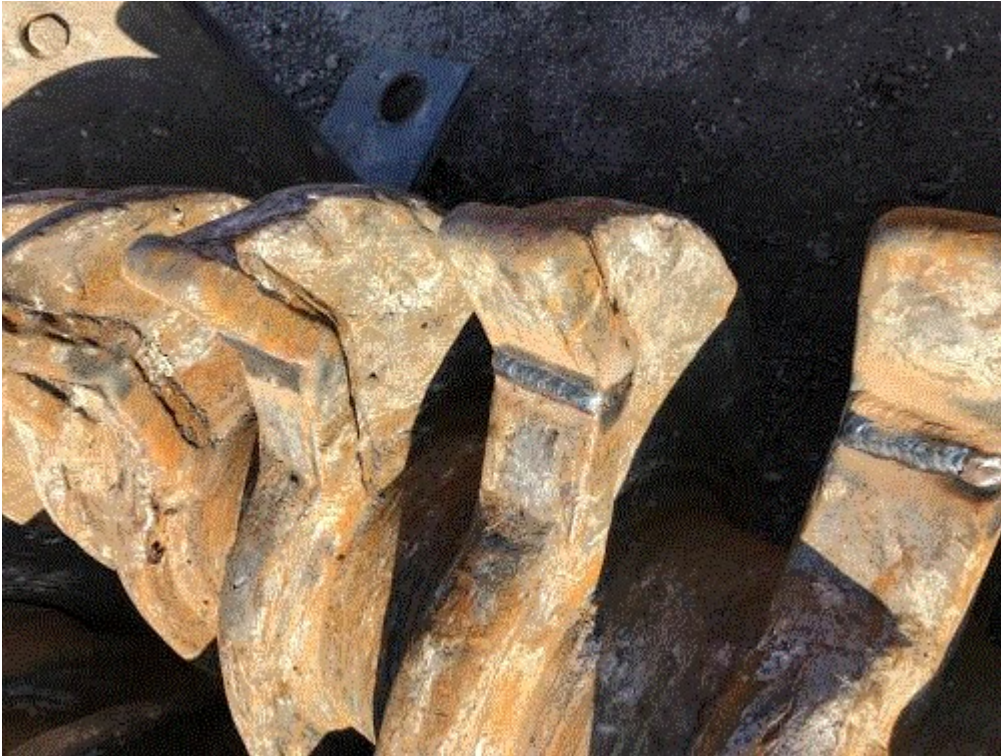
Image 5(fresh welds) : Closer image of fresh welds on the concrete crushing shaft system 9/4/2020
