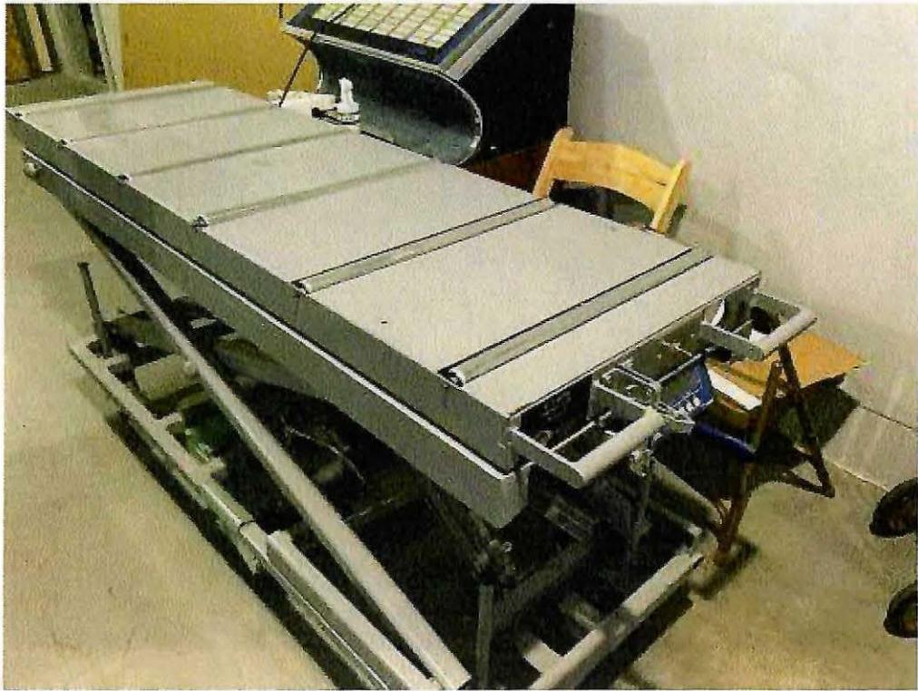
**Image 3(Scale)** : Scale used to weigh charge before being placed into the crematory.
