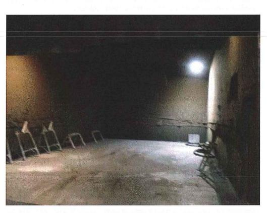
Image 1(Shot Blast) : Enclosed shot blast booth with air recirculation system.
