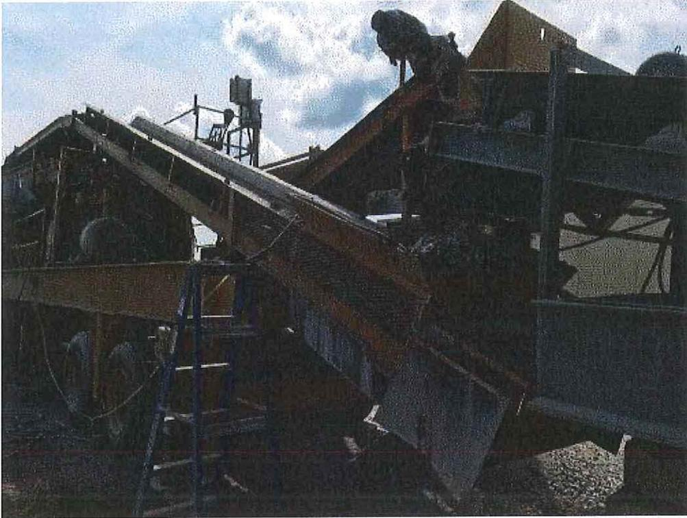
**Image 5(Conveyor) :** Conveyor into cone crusher with water spray attached.
