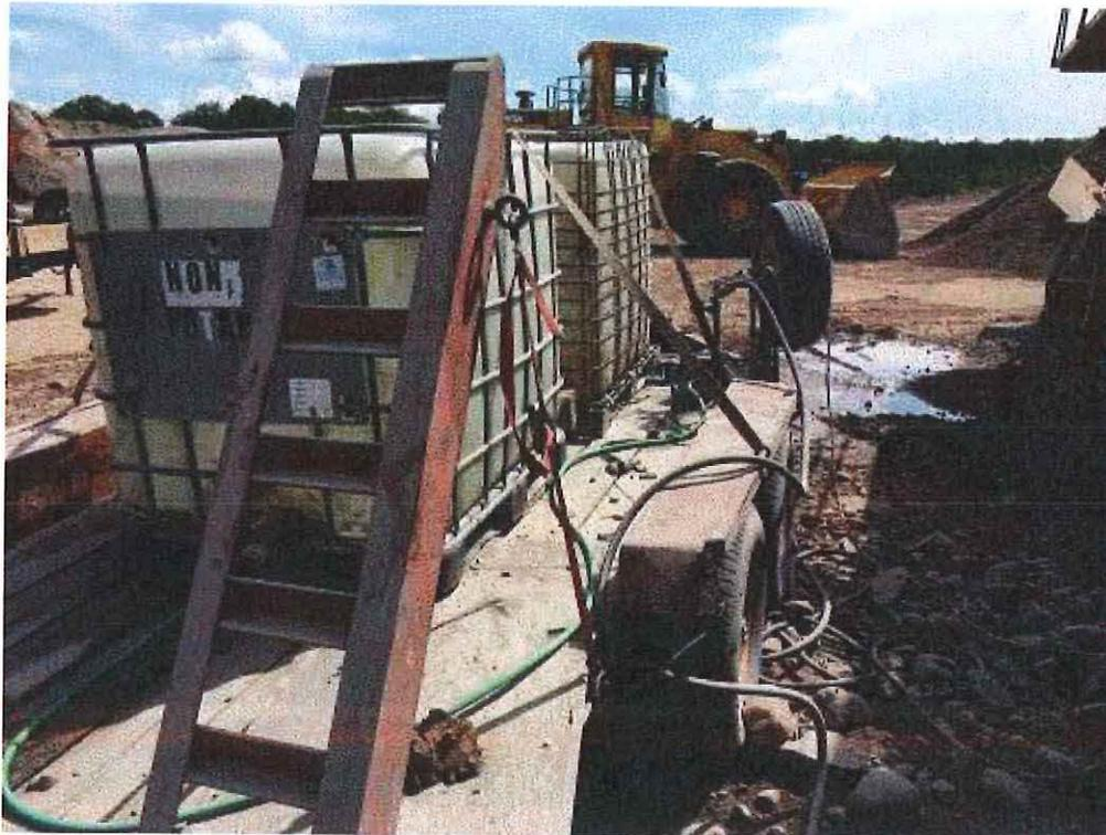
**Image 3(Water Supply)** : Water supply for crushing equipment.
