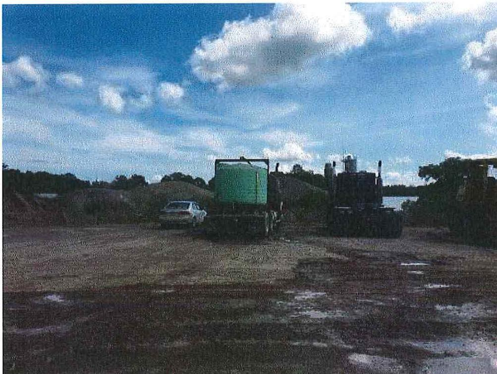
**Image 2(Watering Truck)** : Water truck that is used to control fugitive dust in plant yard.
