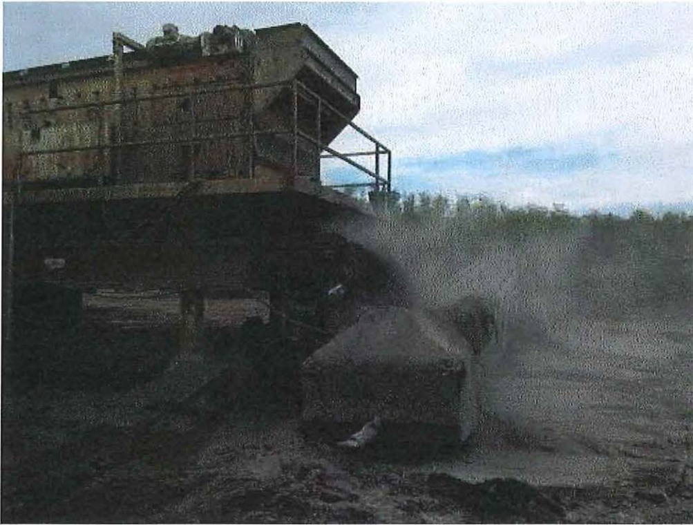
Image 1(Fahrner Crusher 85102) : Fahrner Asphalt Sealers' Crusher with inadequate spray bar and water supply. June 1, 2017.
