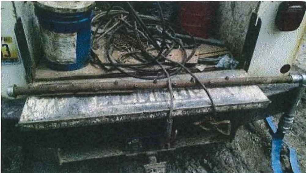
Image 2(New spray bar) : New spray bar for Crusher 85102, prior to installation. June 1, 2017.
