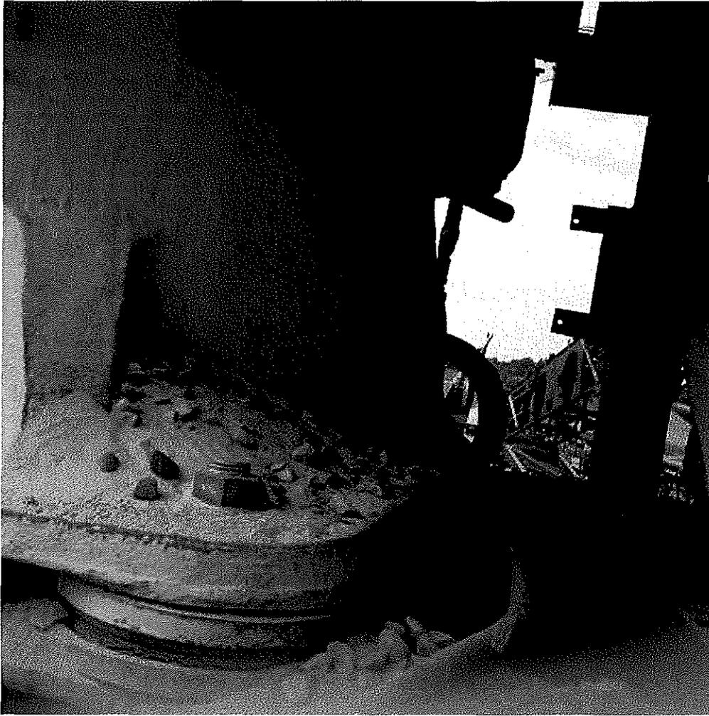
**Image 6(Water Spray)** : Another water injection spot into the crusher
