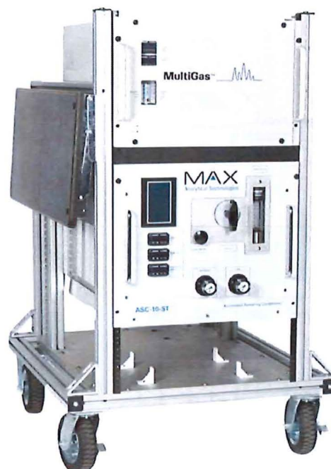
Figure 4.6b: Typical MKS 2030 Multigas FTIR and ASC-10ST Configuration
