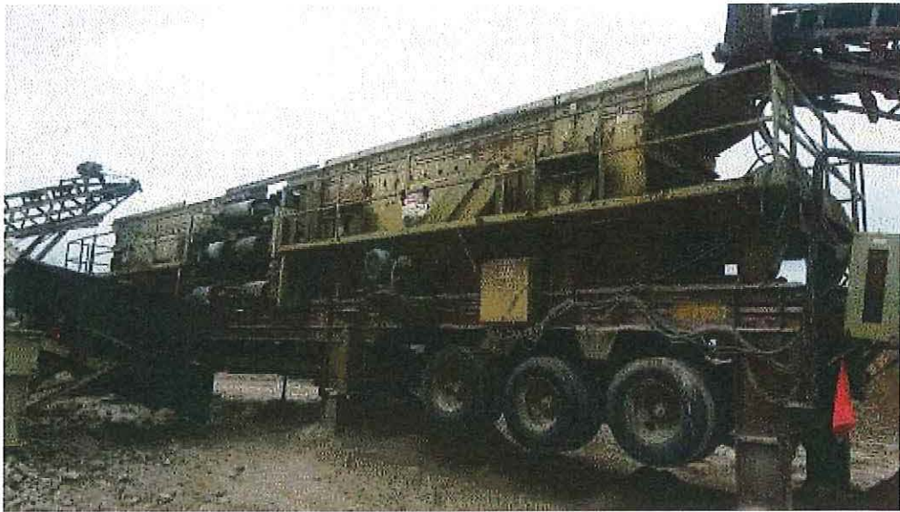
Image 1(CA1) : Telesmith twin screening plant T6x20
