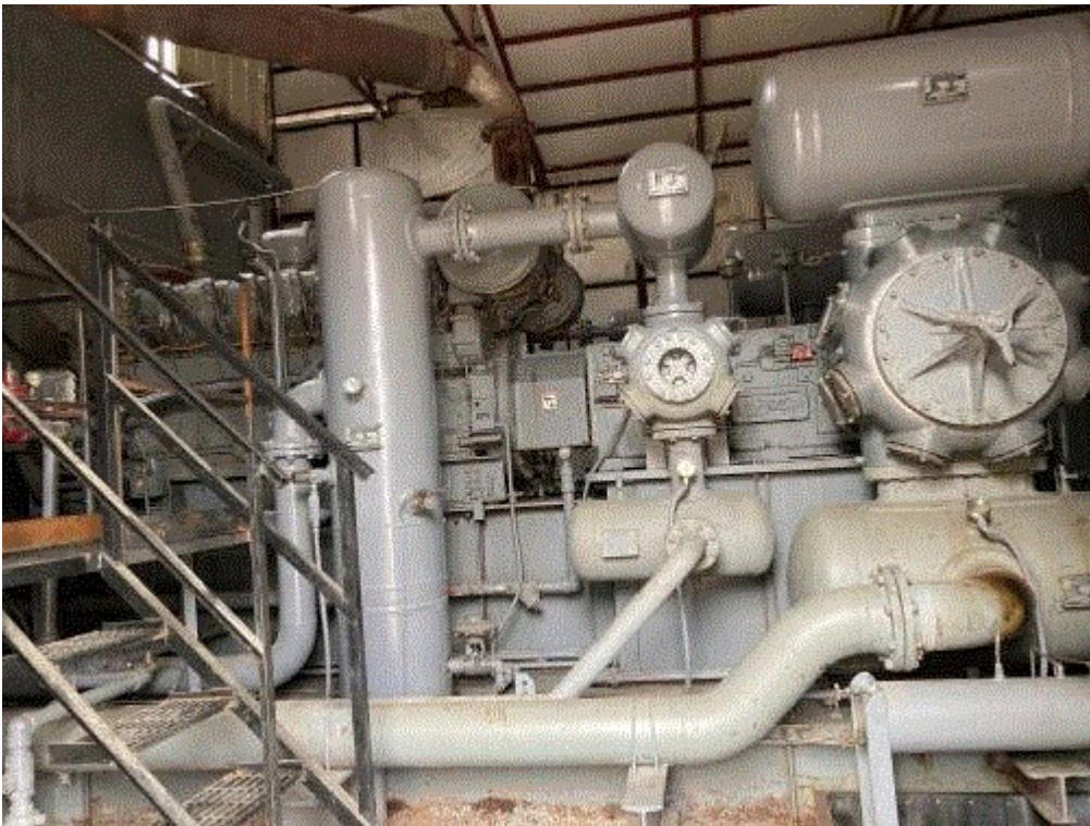
Image 3(CAT3516TA) : 16 Cylinder Engine, 1400 RPM, 1,266 HP
