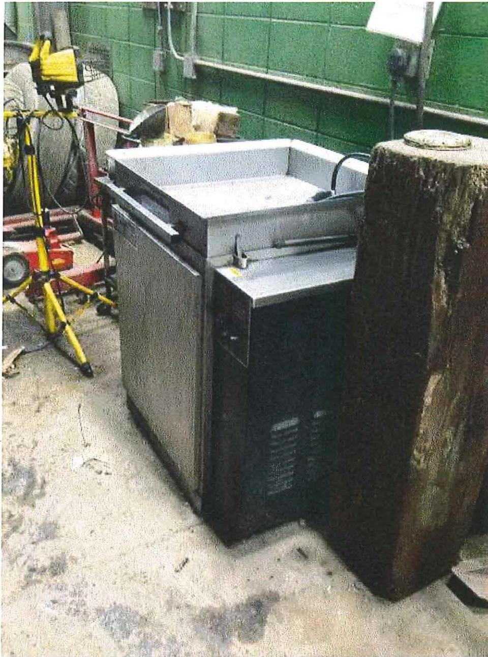
**Image 1(ME1):** Safety Kleen parts washer using aqueous-based solvent which replaced the small parts washer utilizing halogenated solvents.
