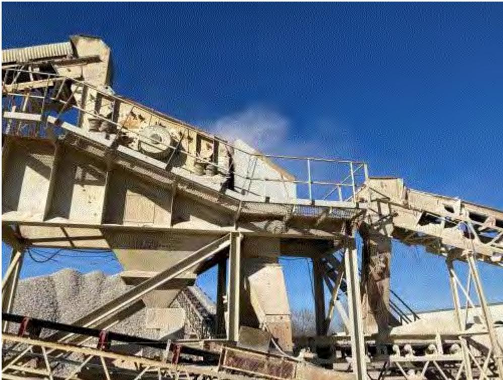
**Image 1(Fugitive Dust 1)** : 5 x 12 Screen (S1) and fugitive dust in excess of 10% standard.
