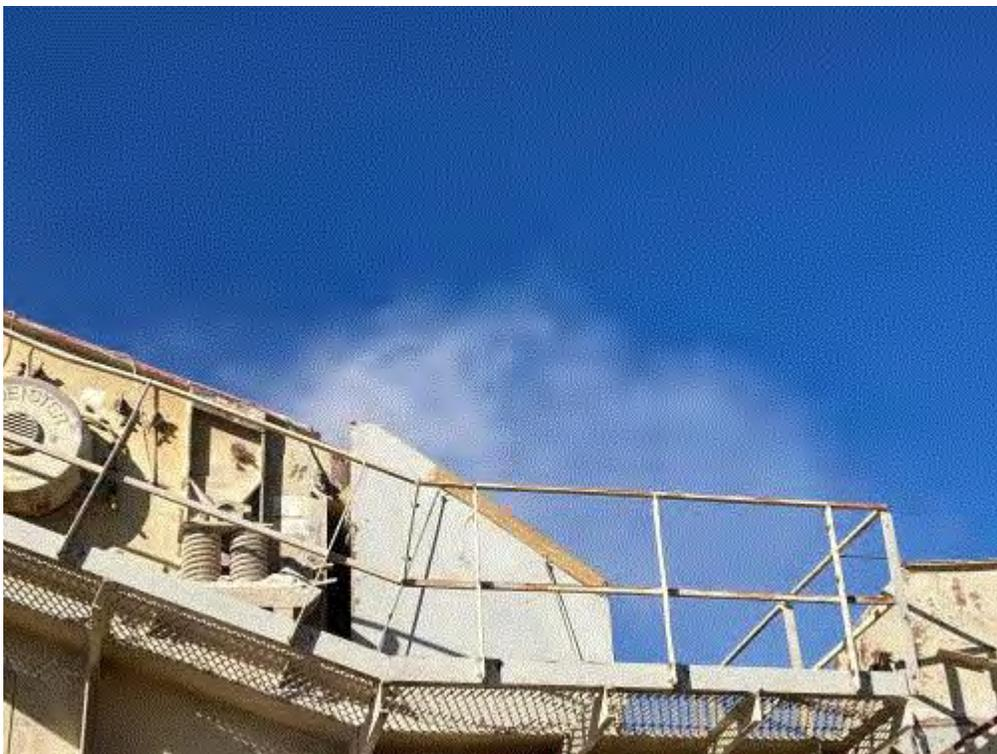
**Image 2(Fugitive Dust 2)** : 5 x 12 Screen (S1) and fugitive dust in excess of 10% standard.
