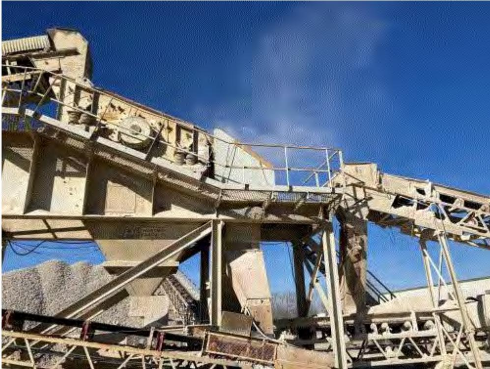
**Image 3(Fugitive Dust 3)** : 5 x 12 Screen (S1) and fugitive dust in excess of 10% standard.
