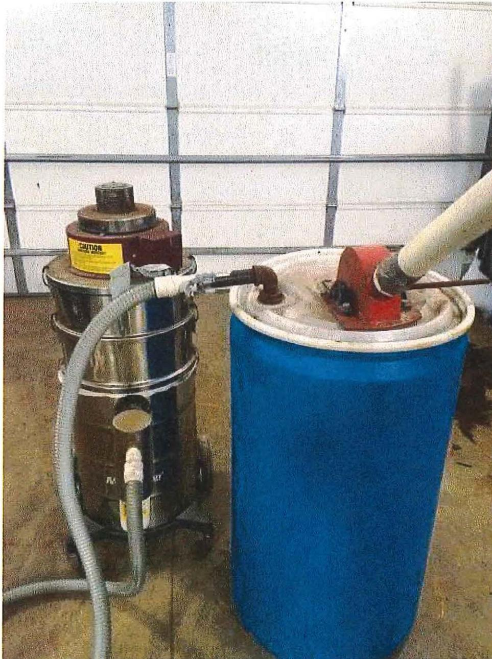
**Image 1(M1) :** Fluorescent bulb crusher w/HEAP vacuum PTI# 117-10
