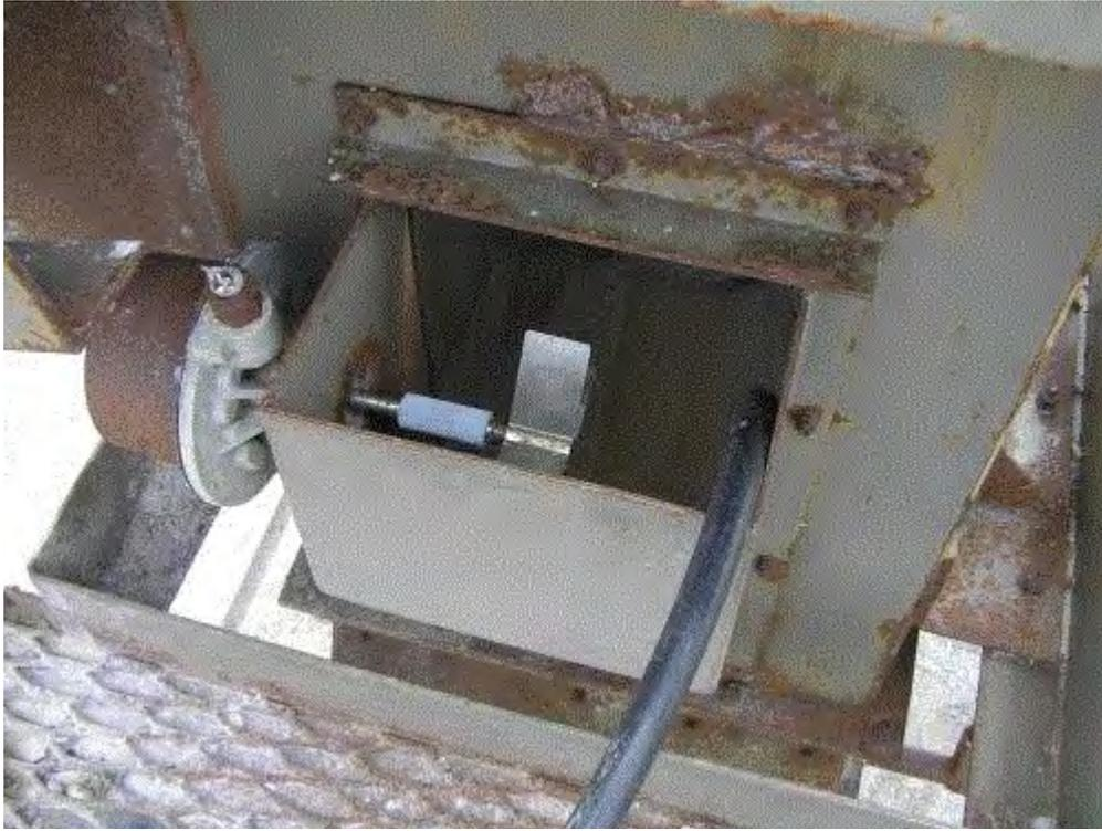
**Image 2(002)** : Hose to supply water to transfer point.
