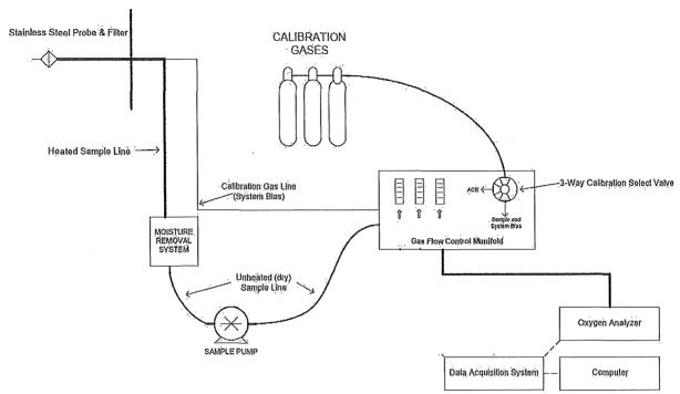
Figure 4-2. USEPA Methods 3A and 7E Sample System
