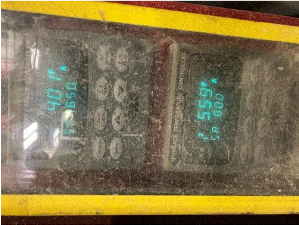
Image 3(Burn off oven temp) : Burn off oven in cool down- top is AB temp, bottom is oven temp.
