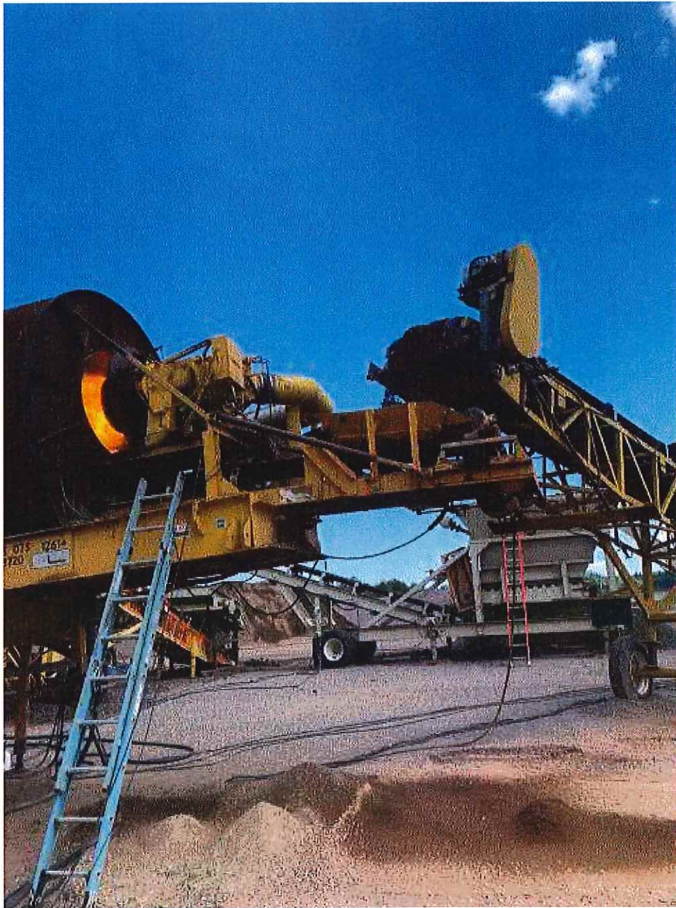
Image 4(Conveyor) : Conveyor to Asphalt Mix Drum
