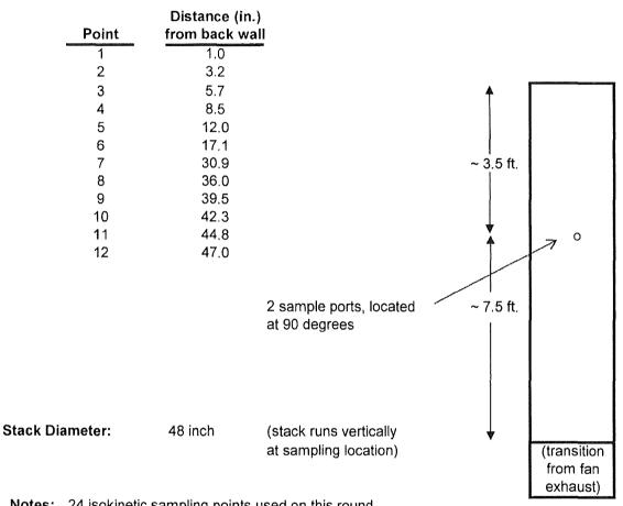
Notes: 24 isokinetic sampling points used on this round stack; 12 points along each of 2 perpendicular traverses. All other gas sampling performed at a single point in the center third of the duct.
