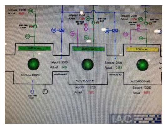
Image 1(Filter Monitoring) : Monitoring for filter pressure drop on FGCOATING2 booths.
