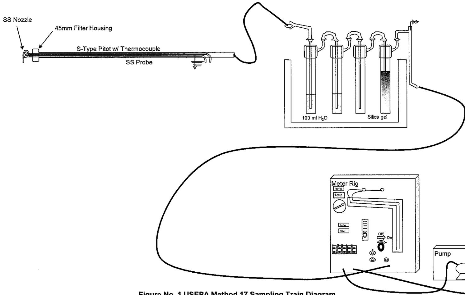
Figure No. 1 USEPA Method 17 Sampling Train Diagram
