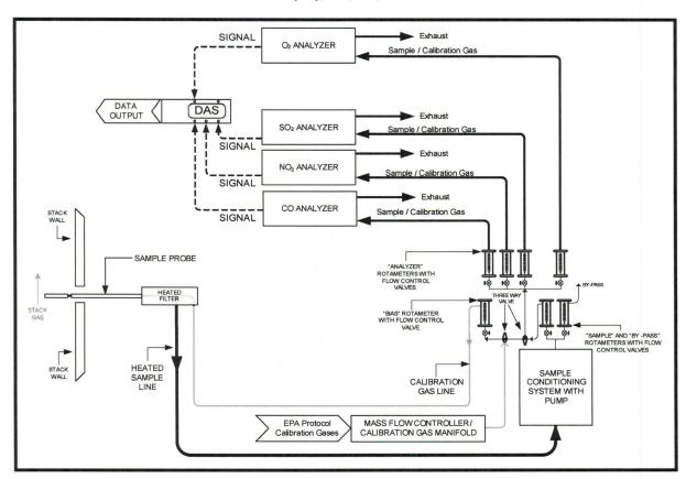
FIGURE 3-2 EPA METHODS 3A (O<sub>2</sub>), 6C, 7E, 10 SAMPLING TRAIN
