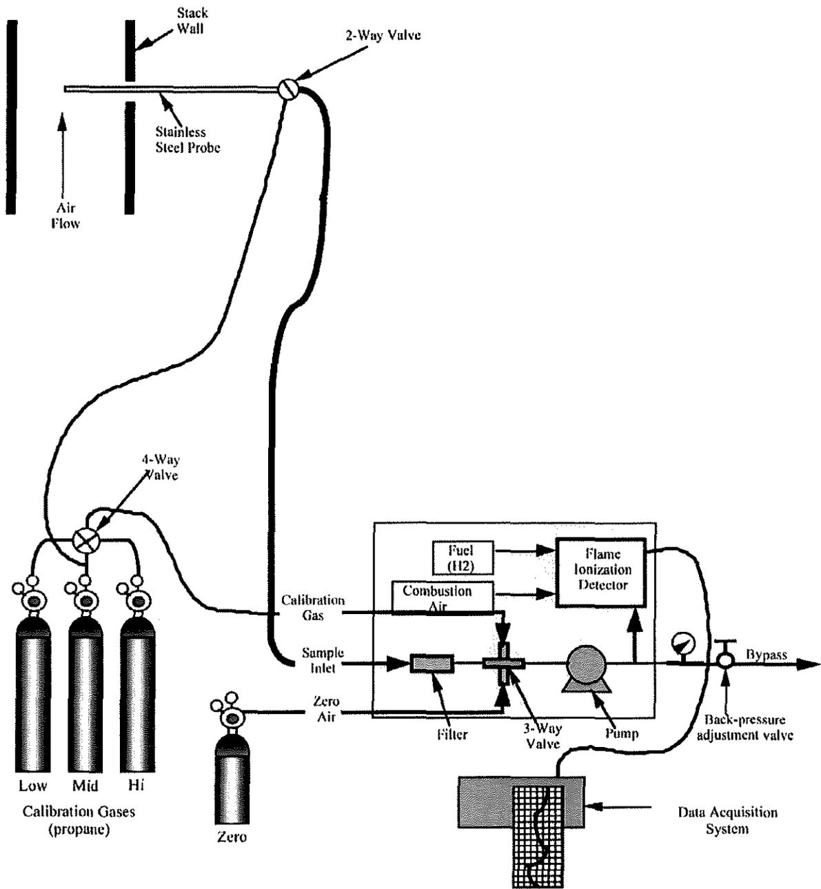
Figure 4-4. USEPA Method 25A Sampling Train
