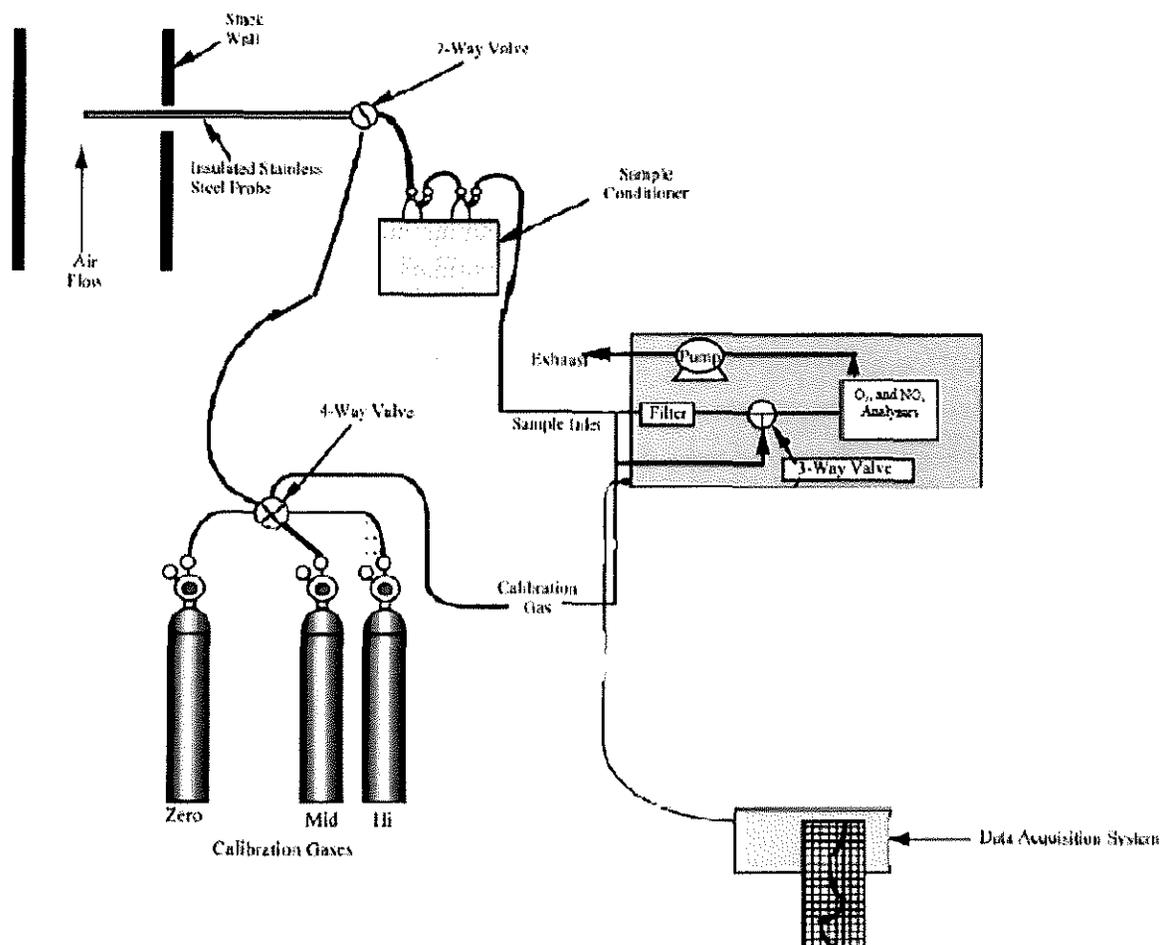
**Figure 4-1. USEPA Methods 3A, 7E, and 10 Sampling Train**
