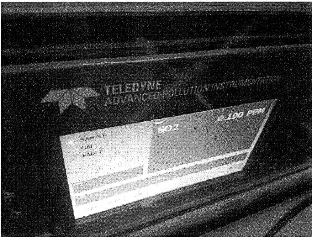
**Image 14(CEMS Control Room) :** SO2 reading of 0.190 ppm
