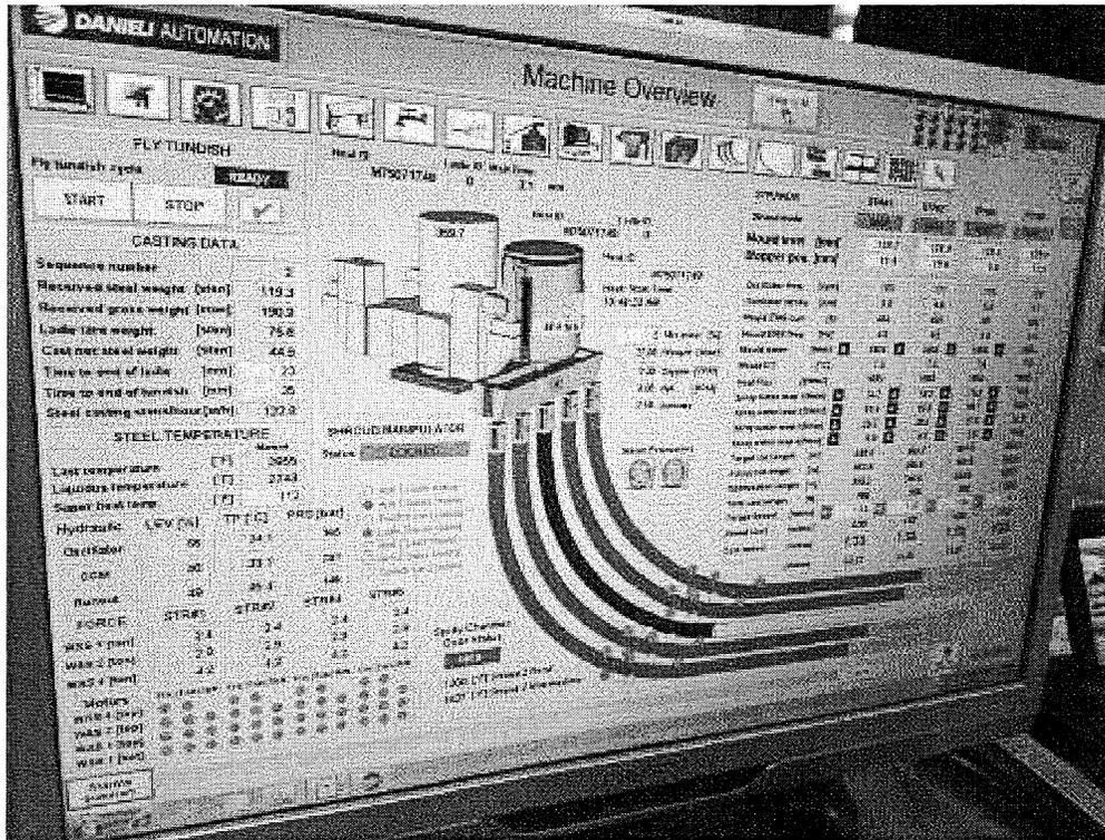
**Image 12(Caster pulpit) :** Caster pulpit control room screen view
