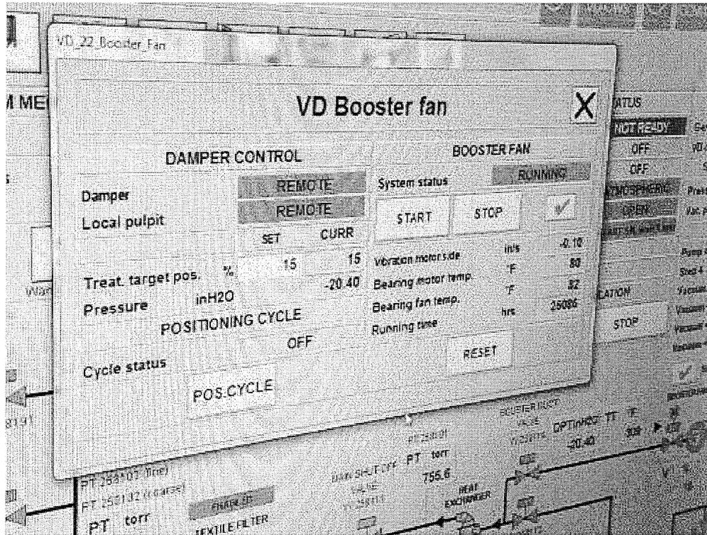
Image 10(VD booster fan) : Vaccum degasser exhaust boost fan screen
