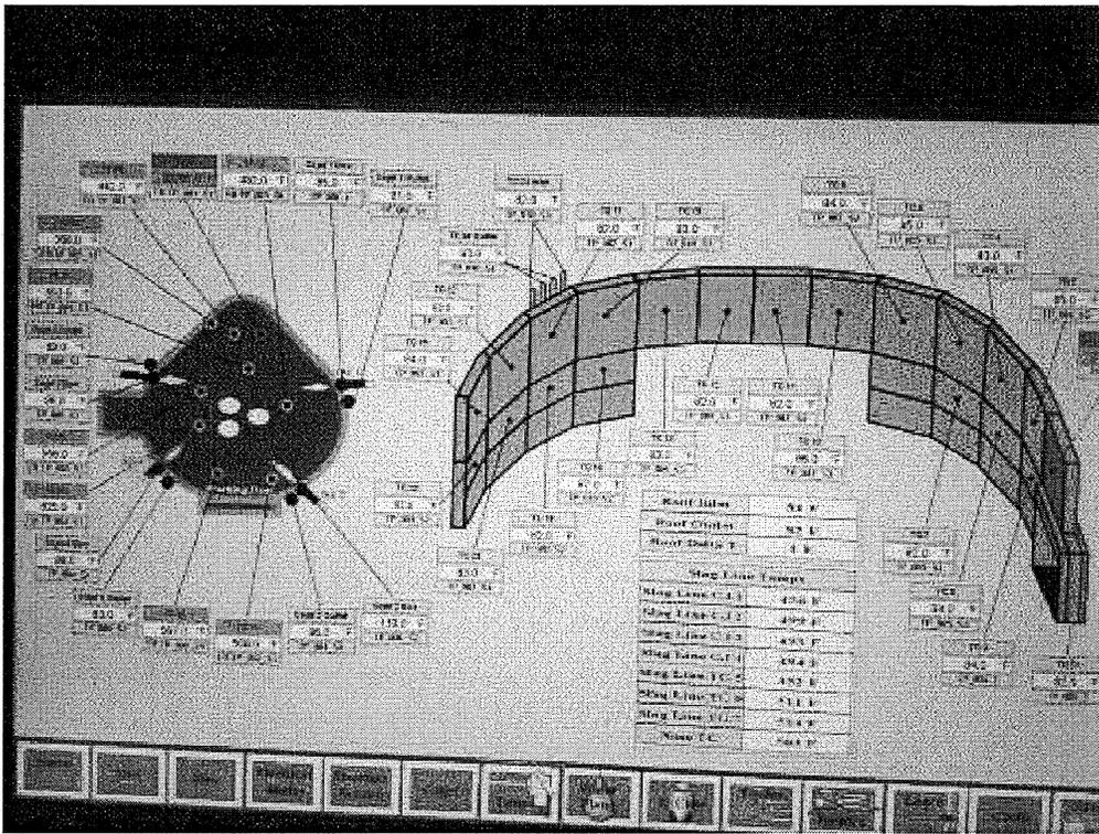
Image 8(EAF view screen) : EAF view screen showing temperatures.
