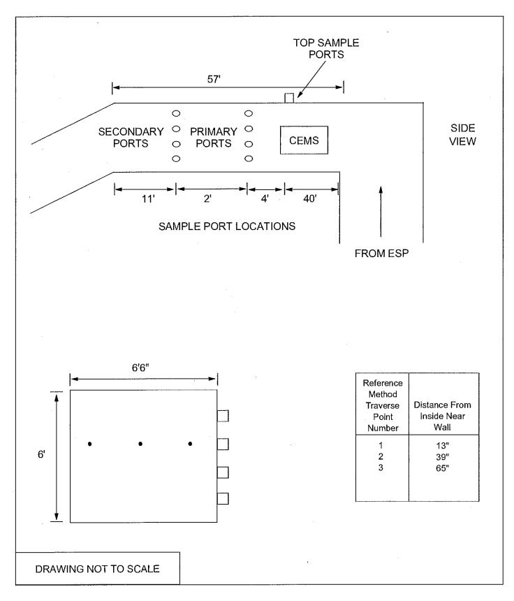
FIGURE 3-1 CEMS AND REFERENCE METHOD TEST LOCATION
