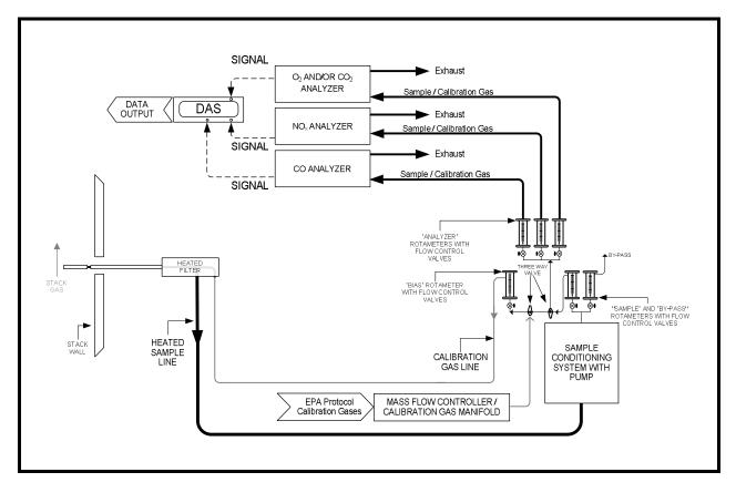
FIGURE 3-1 US EPA METHOD 3A, 7E, AND 10 SAMPLING TRAIN
