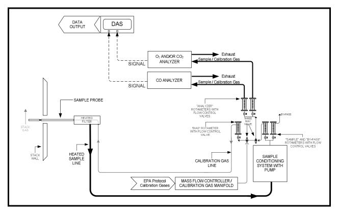
FIGURE 3-2 US EPA METHOD 3A AND 10 SAMPLING TRAIN
