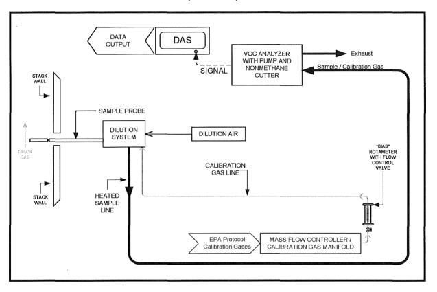
FIGURE 3-2 US EPA METHOD 25A (DILUTION) WITH SAMPLING TRAIN
