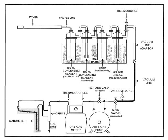
FIGURE 3-1 US EPA METHOD 4 DETACHED SAMPLING TRAIN
