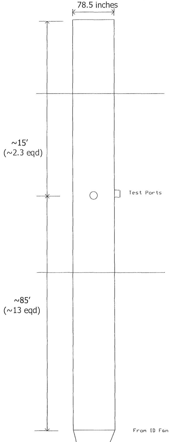
**Figure 5-2: Test Port Location (Outlet Ground Site)**
