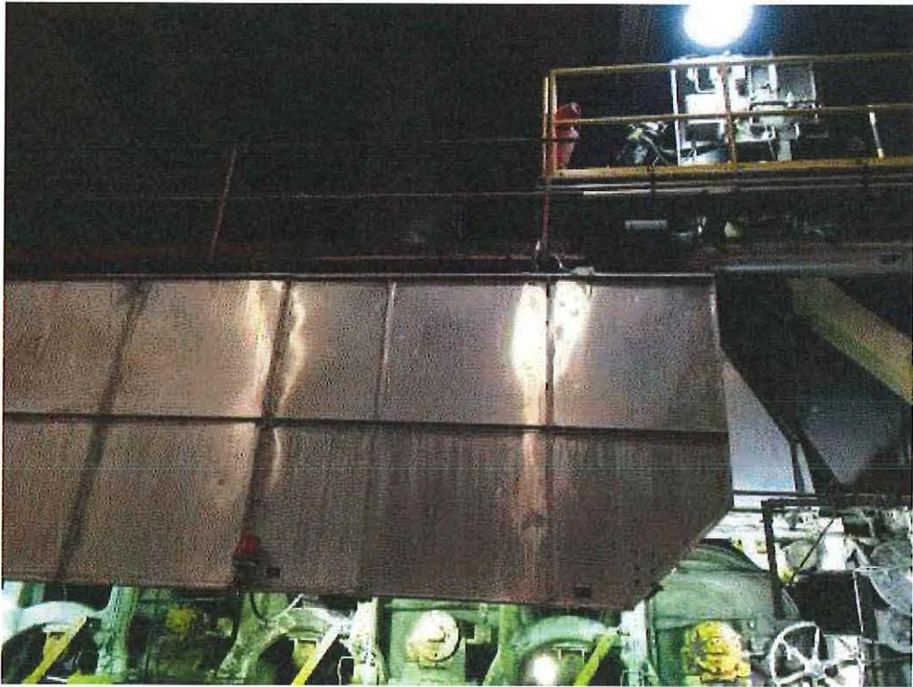
**Image 3(Stack)** : Stack for first dryer of paper machine.
