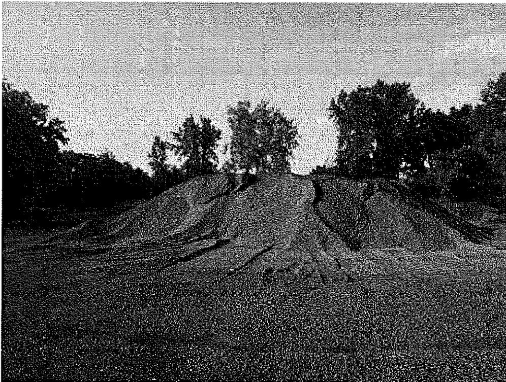
**Image 1(Slag Pile) :** One of 3 slag piles. Raw, middle, fine grade. This one is the middle grade that has already been screened to produce this size of material.
