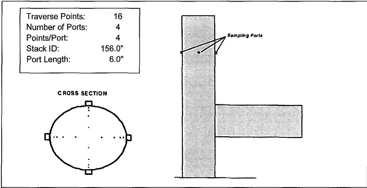
Figure 1-2. Main Stack and Port Diagram
