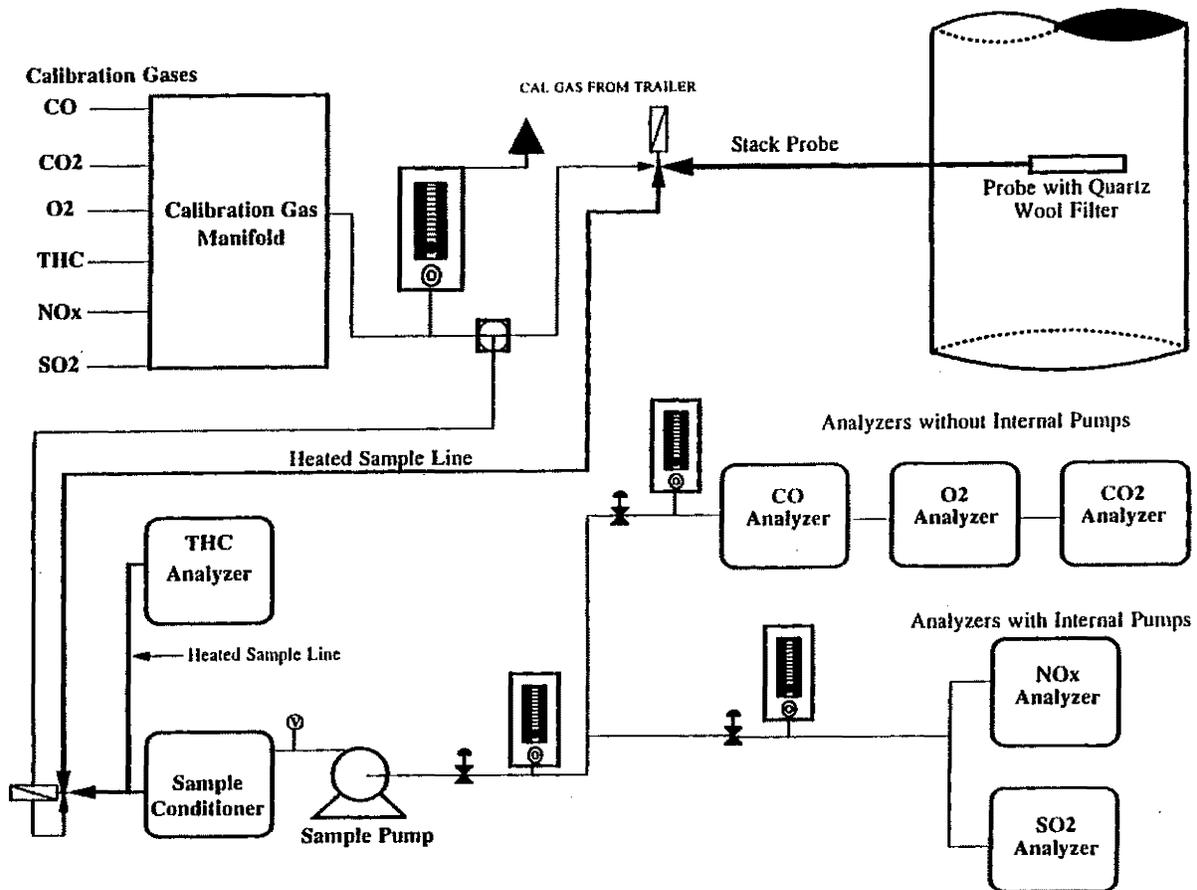
**Figure 3-1. CEM Sample Flow and Calibration System**
