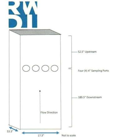
Figure No. 1: Pickle Line Scrubber Exhuast Diagram
