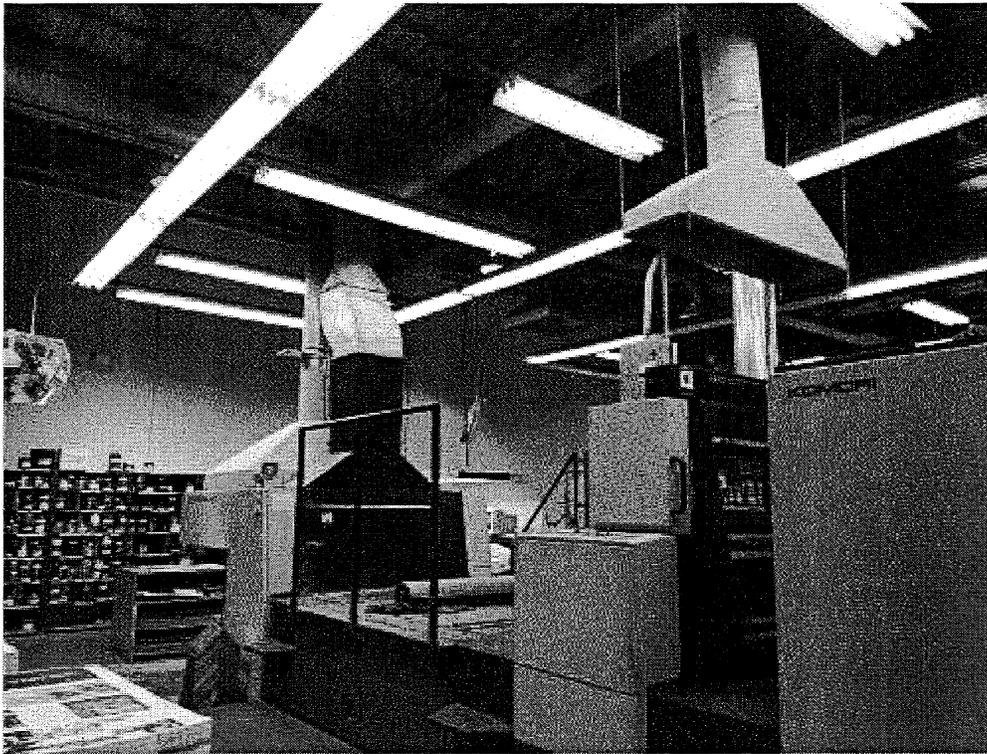
Image 3(Lithographic printer) : Hood collection system from one of the lithographic printers.
