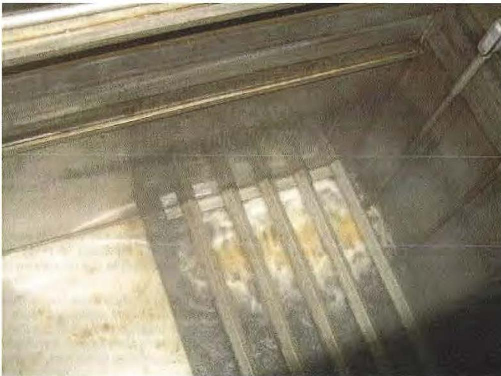
Image 1(001) : NEXT 5408 boiling in solvent sump.
