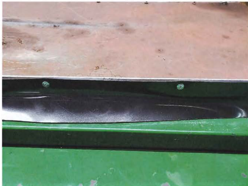
Photo 6: View of rubber shield installed on November 1, 2019 to cover gap between working mode cover and degreaser.
