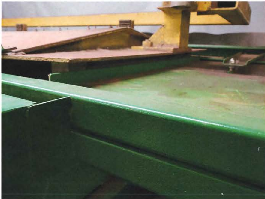
Photo 2: View of approximate 1-inch gap between the working mode cover and degreaser.
