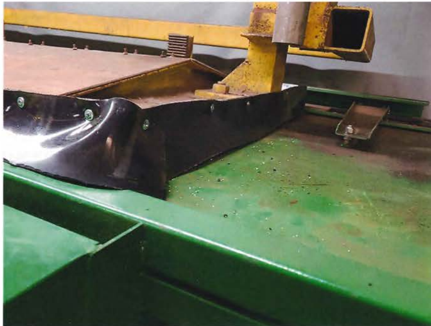
Photo 4: View of rubber shield installed on November 1, 2019 to cover gap between working mode cover and degreaser.
