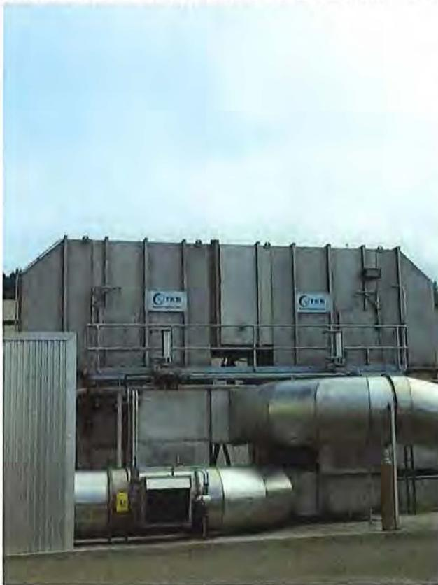
TKS Valves, for distribution into one of two media columns. TKS Valves in conjunction with the **TKS Balanced-Flow Plenums** are the basis for all TKS systems ability to provide continuous 98.0% VOC destruction. The design of these two revolutionary components takes advantage of leak-free construction and minimal flushing volumes. The results provide the user with only high performance and minimized costs.
