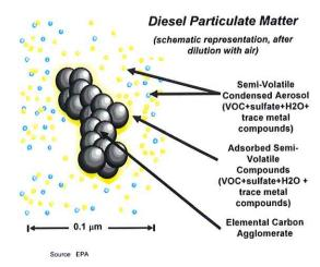
Figure 2 – Formation of PM in Engine Exhaust
