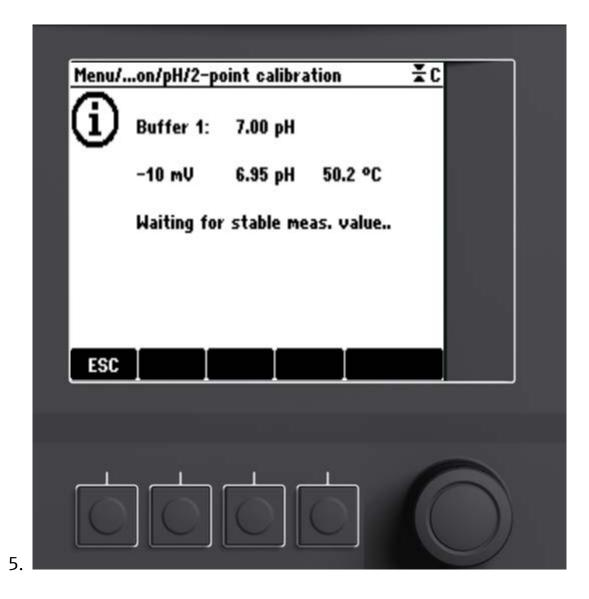
Once finished with the 1<sup>st</sup> buffer, place the sensor in the 2<sup>nd</sup> (usually 4pH), then press "OK"
