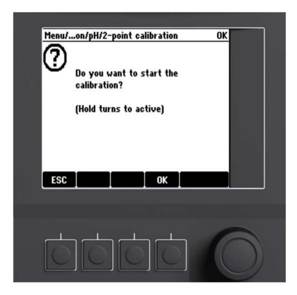
Immerse the sensor in the 1<sup>st</sup> buffer solution (usually 7pH), and press "OK"
