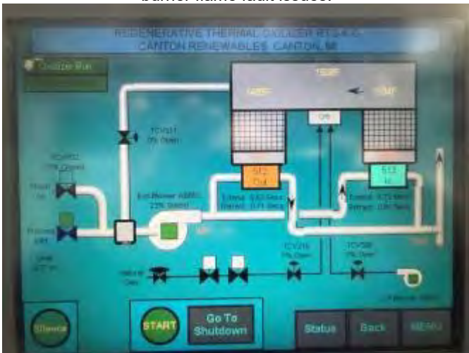
RTO overview screen during online inspection
