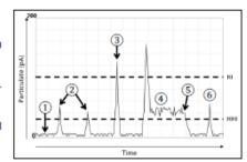
The sharp peaks on the BLDS output represent the brief increase in emission immediately following the baghouse cleaning cycle. For the alarms, a 6-minute average is used to align with the opacity standard, and so the alarm will not activate due to short spikes that are not associated with a cleaning cycle and do not indicate broken bags, such as a spike due to a small amount of PM that accumulates on the duct wall and then breaks free.
