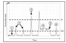
The sharp peaks on the BLDS output represent the brief increase in emission immediately following the baghouse cleaning cycle. For the alarms, a 6-minute average is used to align with the opacity standard, and so the alarm will not activate due to short spikes that are not associated with a cleaning cycle and do not indicate broken bags, such as a spike due to a small amount of PM that accumulates on the duct wall and then breaks free.
