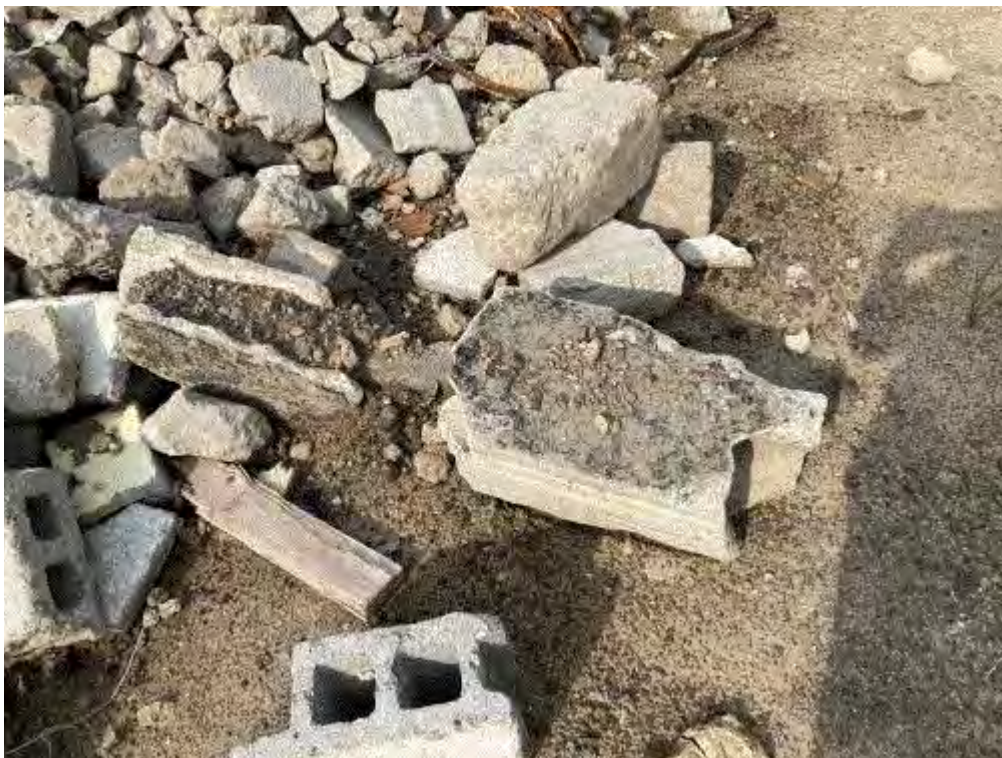
Image 2(Suspect Source Pile) : Pile of concrete mixed with other materials (transformers, scrap metal, etc). This pile is where J. Brown found suspect ACM.
