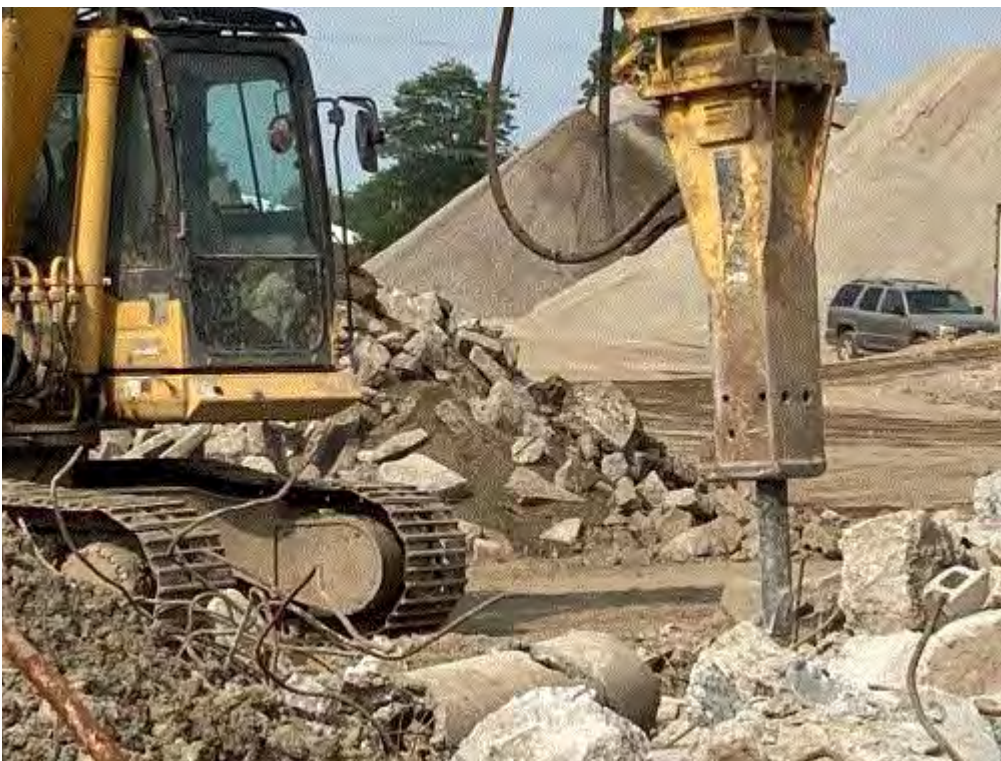
Image 4(Rock Drill) : Rock drill used to break large pieces of concrete into small pieces of concrete.
