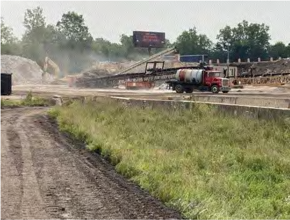
Image 5(Fugitive Dust) : Fugitive dust backlit by sun. Future inspection necessary in the afternoon to allow for a proper viewing angle with respect to the sun. Water truck being used to control fugitive dust from plant yard.
