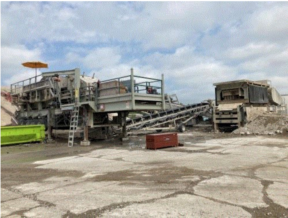
Image 1(001) : Secondary crusher at left and primary crusher at right, with 0% opacity.
