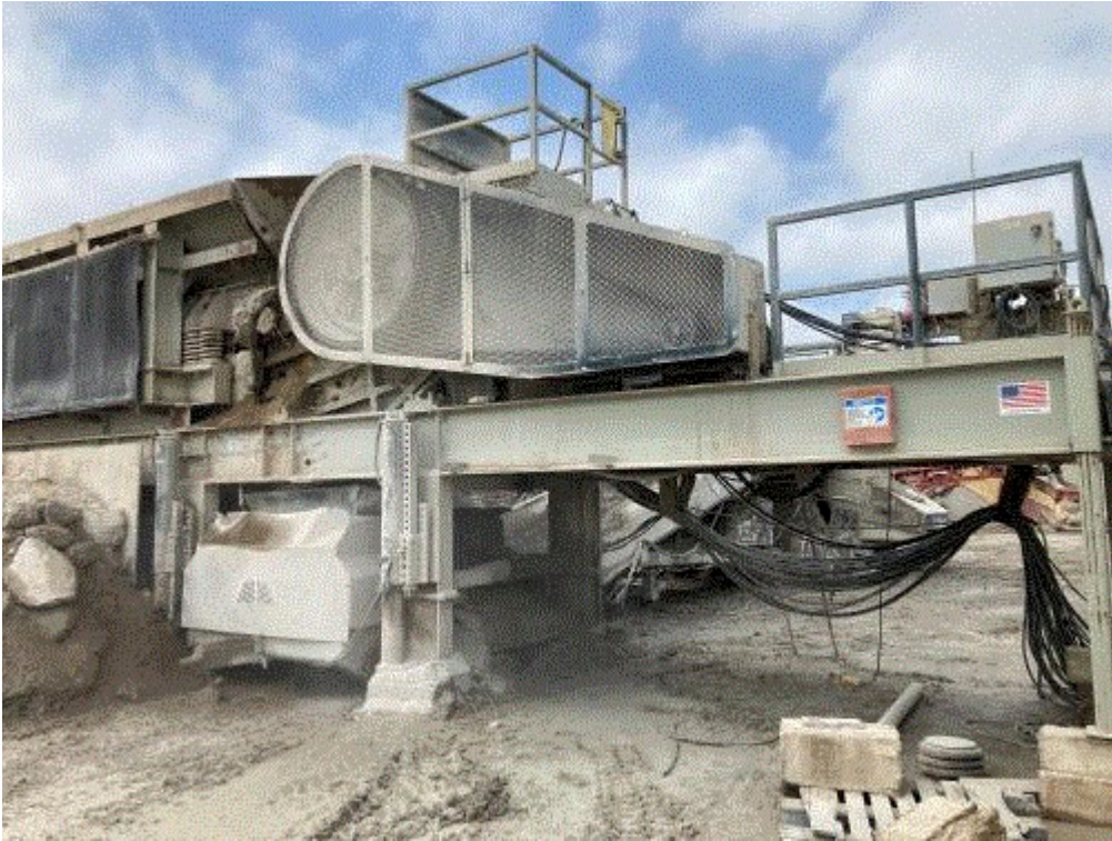
Image 3(003) : Primary crusher, with intermittent opacity of 0-5%, under steel beam just to right of center.
