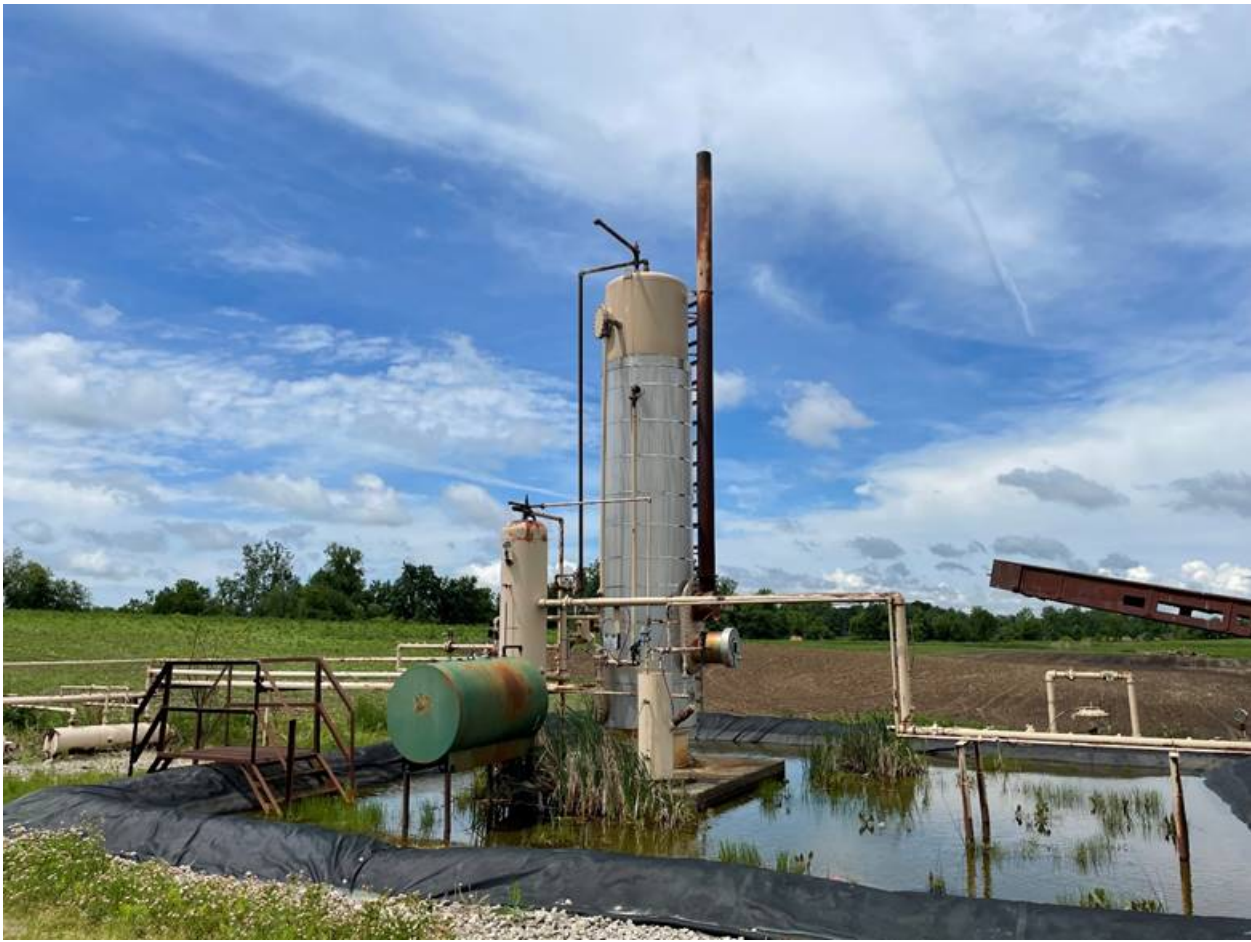
Image 14: Lindeman 1-36 heater treater and line heater.
