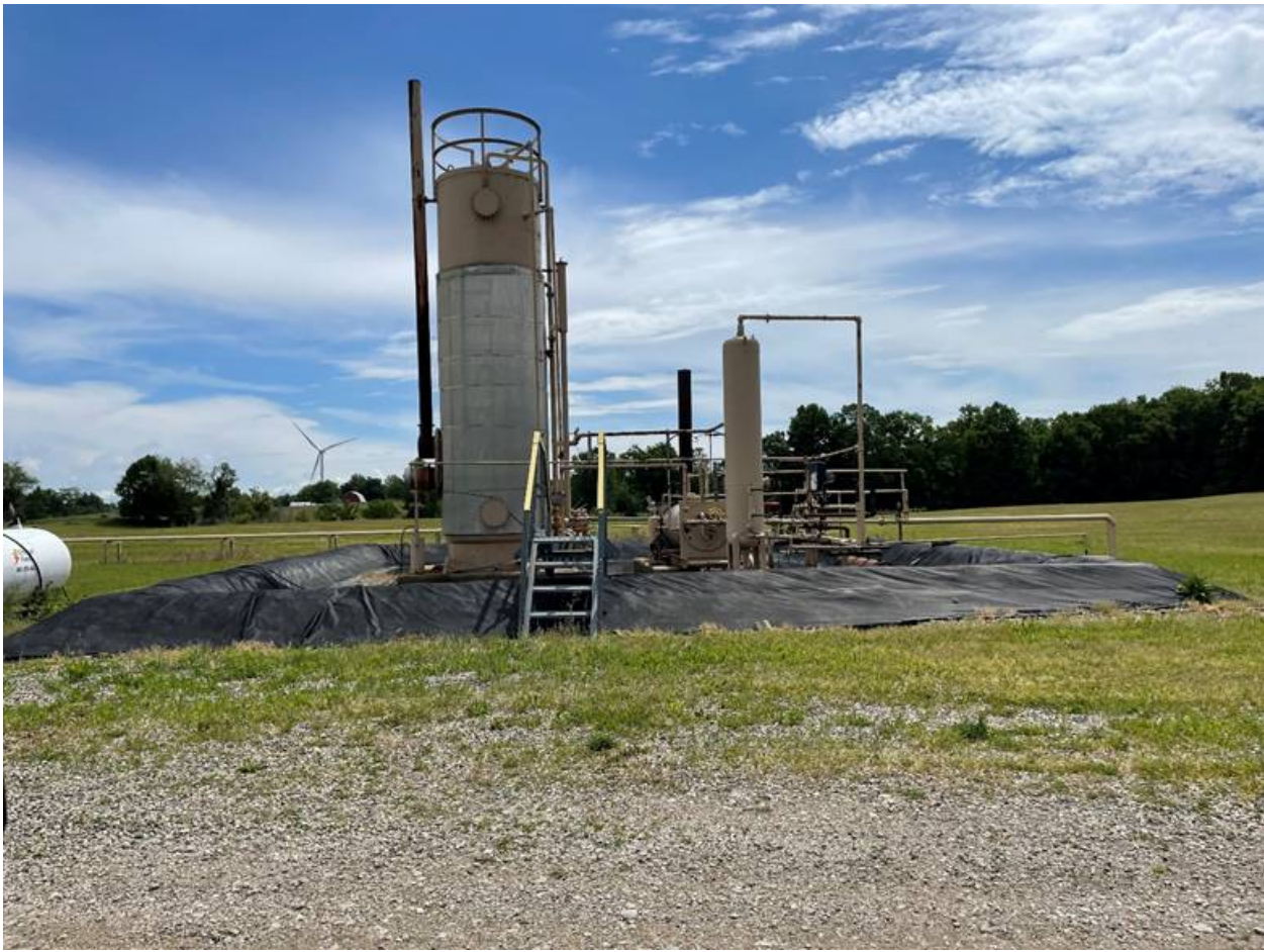
Image 11: Gordon 1-36HD1 heater treater and line heater.
