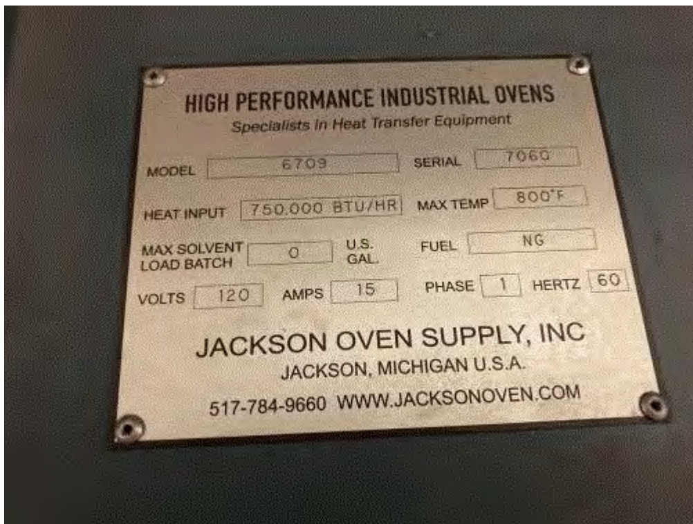
Image 5(PTI 86-20) : Manufacturer's plate information for burn off oven permitted under PTI 86-20. Heat input is a combination of the oven and afterburner heat inputs.
