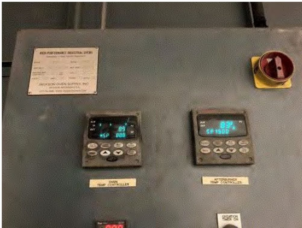
Image 6(PTI 86-20) : Temperature controls (afterburner and oven) for the burnoff oven permitted under PTI 86-20 for continuous monitoring.
