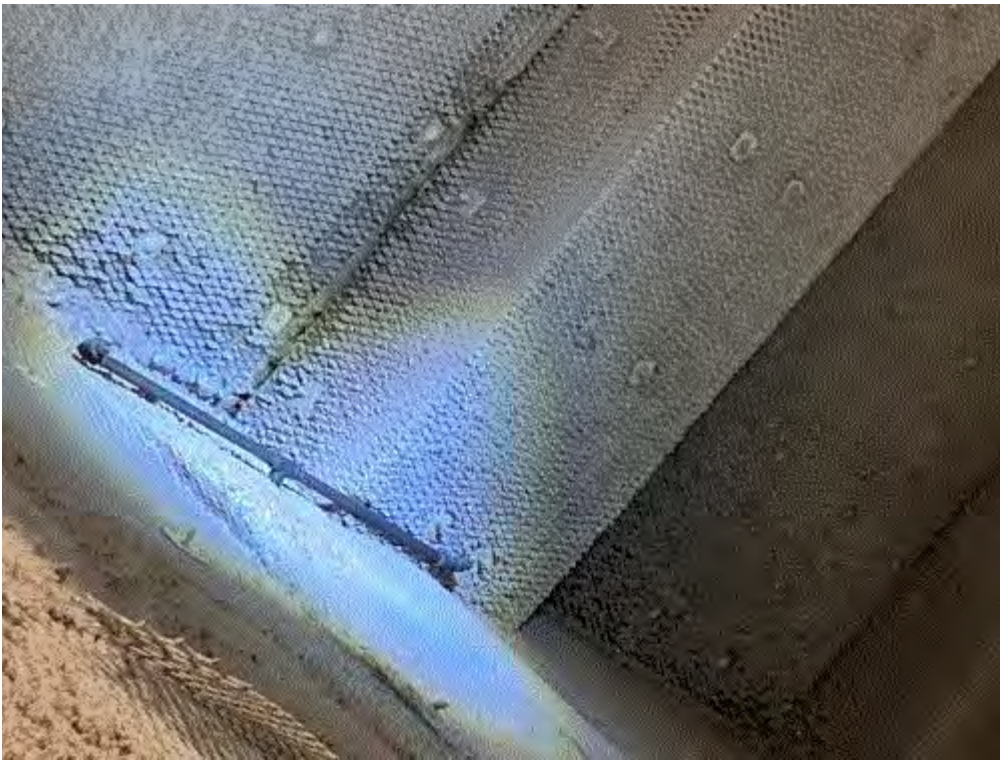
Image 9(Spray Nozzles) : Spray nozzles located in burnoff oven as part of an interlock system to shutdown the oven and bring oven temperature down in the event of a malfunction.
