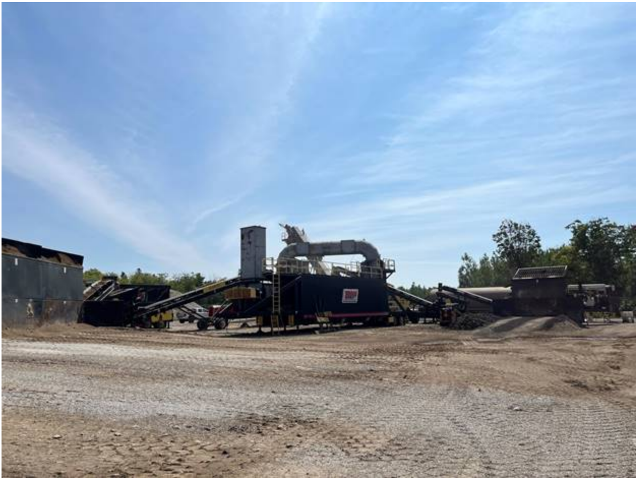
EUHMAPLANT with baghouse and stack installed. No visible emissions observed exiting the baghouse stack.
